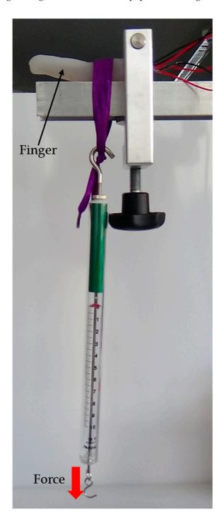
**Figure 11.** Measurement setup to analyze the force sensor. Force is applied to the proximal sensor using a flexible (purple) band.
