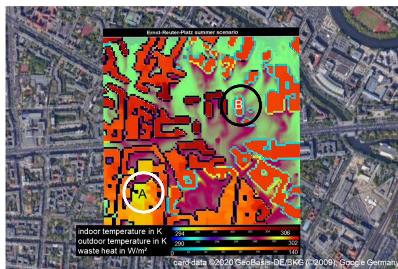
Figure 15. Excerpt from an urban climate simulation. The Ernst-Reuter-Platz in Berlin connects five urban street canyons and is surrounded by high-rise buildings. The simulation runs with a resolution of 1\text{ m} \times 1\text{ m} \times 1\text{ m} . The outdoor temperature is around 24\text{ }^{\circ}\text{C} in the summer scenario. The graph shows the indoor and temperature, and the anthropogenic waste heat at the outside surface, depending on the air conditioning concept. Façade elements with no anthropogenic waste heat (i.e., buildings with passive cooling in summer) are shown in black. From a PALM simulation, run by Leibniz University Hannover, cited by [53].
