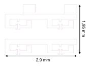
Figure A.4: Layout for printed crossbar PUF core signal routing layer.
