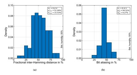
Figure 6.11: PE-based DiffC-PUF uniqueness and bit aliasing. (a) PE-based DiffC-PUF uniqueness.
