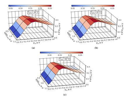
Figure 5.16: Standard deviation s of V<sub>out</sub> over T<sub>amb</sub> = {−20 °C, 23 °C, 60 °C}, V<sub>in</sub> and VDD<sub>core</sub>, visualized as surface plot. (a) Surface plot at −20 °C. (b) Surface plot at 23 °C. (c) Surface plot at 60 °C. Adapted from [129], © 2019 IEEE.
