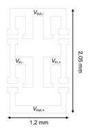
Figure A.2: Full-wave rectifier signal routing layer layout.
