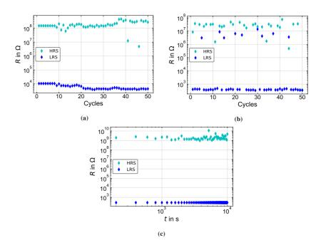
Figure 4.8: Endurance and retention test results of the printed device. (a) Endurance test using DC sweep cycling over 50 cycles. (b) Endurance test using pulse voltage cycling over 50 cycles. (c) Retention test over 10<sup>4</sup> s time period over the HRS and LRS, respectively. Adapted from [203], © 2021 AIP Publishing.
