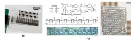
Figure 2.4: Advanced circuits based on printed TFTs. (a) Printed OTFT-based address decoder and ferroelectric memory on flexible substrate, connected with rigid printed circuit board (PCB) [88]. Reproduced under CC BY-NC-ND 3.0 license, https://creativecommons.org/licenses/by-nc-nd/3.0/. (b) Electrochemically-gated transistors deployed in addressing circuitry for an integrated electrochromic display [93]. Reproduced under CC BY 4.0 license, https://creativecommons.org/licenses/by/4.0/.
