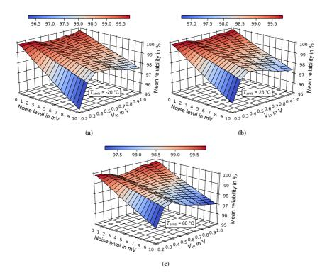
Figure 5.17: DiffC-PUF reliability over noise levels and temperature, visualized as surface plot. (a) Reliability surface plot at -20 °C. (b) Reliability surface plot at 23 °C. (c) Reliability surface plot at 60 °C. Adapted from [129], © 2019 IEEE.
