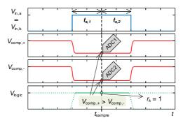
Figure 6.2: Schematical readout timing setup for the voltage levels and the corresponding output bit. Adapted from [138] under CC BY 4.0 license, https://creativecommons.org/licenses/by/4.0/.
