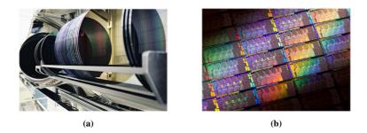
Figure 1.1: Exemplary images for Si-based electronics from wafer to IC. (a) Multiple bare silicon wafers. Source: Infineon Technologies. (b) ICs in the form of an Intel "Sandy Bridge" microprocessor architecture, based on 32 nm technology node, on processed wafer. Source: Intel Free Press, reproduced under CC BY-SA 2.0 license, https://creativecommons.org/licenses/by-sa/2.0/.
