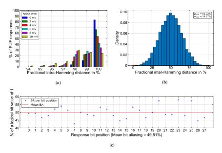
Figure 5.19: DiffC-PUF reliability uniqueness and bit aliasing at  $V_{in} = 0.4$  V. (a) Reliability plotted over the intra-FHD. (b) Uniqueness plotted over the inter-FHD. (c) Bit aliasing plotted over each response bit position, including mean bit aliasing. Adapted from [129], © 2019 IEEE.
