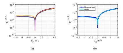
**Figure 5.2:** Near-zero threshold voltage, diode-connected EGT I - V curves plotted on semilogarithmic scale over the absolute drain current and EKV model fit. (a) Four measured diode-connected near-zero  $V_{\text{th}}$  EGT I - V curves with a channel width  $W_{\text{T}} = 200 \,\mu\text{m}$ and length  $L_{\text{T}} = 90 \,\mu\text{m}$  at RH = 60%. (b) Fitted EKV model curve over one of the measured diode-connected EGT. Adapted from [80], © 2020 IEEE.
