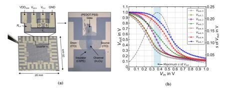
Figure 5.22: PE-based DiffC-PUF core on glass substrate. (a) Photograph of the fabricated DiffC-PUF core. (b) Measured inverter transfer curves, including the standard deviation of the incorporated inverters V<sub>out</sub>. Adapted from [129], © 2019 IEEE.
