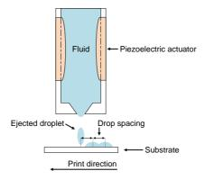
Figure 2.2: Schematic for a DoD piezo-inkjet printhead ejecting a droplet on a carrier substrate within a defined drop spacing.
