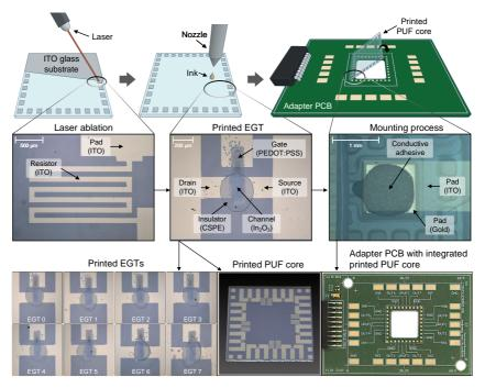
Figure 6.8: Fabrication and integration workflow of the PE-based DiffC-PUF core on the adapter PCB, from left to right. Furthermore, additional images are shown, such as microscopic images of eight EGTs on a printed PUF core, a standalone printed PUF core on glass substrate and the integrated PUF core on the adapter PCB. Adapted from [200] under CC BY 4.0 license, https://creativecommons.org/licenses/by/4.0/.
