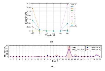
Figure 6.7: Measured Si-based DiffC-PUF bit errors. (a) BE of 10 DiffC-PUF cores, visualized over T<sub>amb</sub>. (b) BE of 30 DiffC-PUF cores over two deployed control logic boards (A and B). Adapted from [138] under CC BY 4.0 license, https://creativecommons.org/licenses/by/4.0/.
