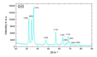
Figure 4.4: X-ray powder diffraction results of the poly-crystalline ZnO film, formed from the inkjetprinted zinc-nitrate precursor salt. Adapted from [203], © 2021 AIP Publishing.
