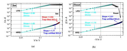
Figure 4.9: Double-logarithmic I - V plot for conduction mechanism investigation. (a) Set process investigation including the linear fitted curves and corresponding slopes over different voltage regions. (b) Reset process investigation, including the linear fitted curves and corresponding slopes, over different voltage regions. Adapted from [203], © 2021 AIP Publishing.
