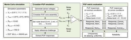
Figure 5.8: Printed crossbar PUF simulation methodology including noise level allocation and simulation parameter. Adapted from [129], ©2019 IEEE.
