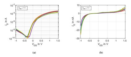
Figure 4.2: Measured transfer curves and corresponding gate leakage of five EGTS with a channel width  $W_T = 200 \,\mu\text{m}$  and length  $L_T = 60 \,\mu\text{m}$  at  $V_{\text{DS}} = 1 \,\text{V}$  and RH = 50 %. (a) Transfer curves of the measured EGTs, with  $I_{\text{D}}$  plotted in logarithmic scale. (b) The corresponding gate leakage currents.
