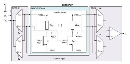
Figure 5.14: System architecture of the DiffC-PUF, including the inverter-based PUF core and the Si-based control logic. Adapted from [138] under CC BY 4.0 license, https://creativecommons.org/licenses/by/4.0/.
