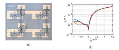
Figure 5.12: Fabricated PUF crossbar and measured device characteristics. (a) Stitched microscopic image of a fabricated  $2 \times 2$ -cells, diode-connected EGT-based printed crossbar PUF at  $5 \times$  optical magnification. (b) Addressed crossbar cells I - V curves, measured at RH = 50 % on semi-logarithmic scale. Adapted from [219], © 2021 IEEE.
