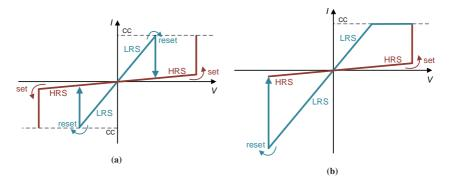
Figure 3.3: Typical switching behavior of memristors, including compliance current for current limiting, when the device switches from HRS to LRS. (a) Unipolar device switching. Set and reset voltages have the same polarities. (b) Bipolar device switching. Set and reset voltages require opposite polarities.
