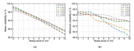
Figure 5.21: DiffC-PUF reliability over  $V_{in} = \{0.35 \text{ V}, 0.375 \text{ V}, ..., 0.45 \text{ V}\}$  and NL. (a) Mean reliability. (b) Minimum reliability. Adapted from [129], © 2019 IEEE.
