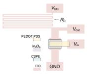
Figure 5.13: Inverter incorporating resistive ITO strip and EGT, including probing pad labels.
