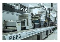
Figure 2.1: Pilot printing line "Gallus RCS 330", using conventional printing methods for PE. Source: Innovationlab GmbH.
