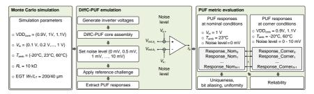
Figure 5.15: DiffC-PUF simulation methodology including noise level allocation and simulation parameter. Adapted from [129], ©2019 IEEE.
