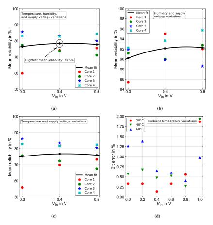
Figure 6.10: PE-based DiffC-PUF reliability over  $V_{in} = \{0.3 V, 0.4 V, 0.5 V\}$  and bit errors over  $V_{in} = \{0 V, 0.2 V, ..., 1 V\}$ . (a) Reliability including variation in  $T_{amb}$ , RH and VDD<sub>core</sub>. (b) Reliability including variation in RH and VDD<sub>core</sub>. (c) Reliability including variation in  $T_{amb}$  and VDD<sub>core</sub>. (d) Bit error metric over  $T_{amb}$ . Adapted from [200] under CC BY 4.0 license, https://creativecommons.org/licenses/by/4.0/.
