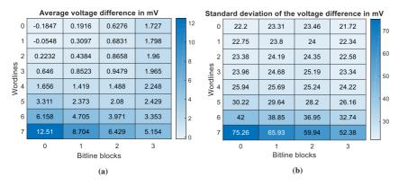
Figure 5.9: Voltage difference ( $\Delta V_{sen}$ ) investigations. (a) Average voltage difference of each bitline block. (b) Standard deviation of the voltage difference.
