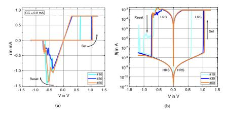
Figure 4.5: I - V curves of the inkjet-printed memristor, which shows a bipolar-switching behavior. For the set process, a compliance current of 0.8 mA is used. Furthermore, ECM-cell type switching behavior is observable. (a) I - V curves on a linear scale, showing cycle number ten, 30 and 50. (b) I - V curves on a semi-logarithmic scale, showing cycle number ten, 30 and 50. Adapted from [203], © 2021 AIP Publishing.
