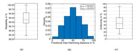
Figure 6.6: Measured Si-based DiffC-PUF metrics. (a) Reliability of 10 DiffC-PUF cores, visualized as boxplot. (b) Uniqueness plotted over the inter-FHD, including 30 DiffC-PUF cores. (c) Uniformity, visualized as boxplot, incorporating 30 Sibased DiffC-PUF cores. Adapted from [138] under CC BY 4.0 license, https://creativecommons.org/licenses/by/4.0/.
