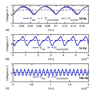
Figure 5.4: Frequency dependency of the full-wave rectifier. (a) Rectifier output voltages V<sub>out</sub>, V<sub>out</sub>, smooth and V<sub>out,sim</sub>. (b) Rectifier output voltage at 1 kHz. (c) Rectifier output voltage at 10 kHz. Adapted from [80], © 2020 IEEE.
