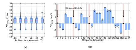
Figure 6.5: Si-based DiffC-PUF comparator input voltage differences  $\Delta V_{comp}$ . (a)  $\Delta V_{comp}$  of ten PUF cores over temperature. (b)  $\Delta V_{comp}$  per response bit of one selected PUF core (no. 20). Adapted from [138] under CC BY 4.0 license, https://creativecommons.org/licenses/by/4.0/.
