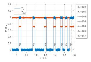
Figure 6.4: Exemplary input and output voltages of inverter number six of an arbitrary Si-based DiffC-PUF core. The corresponding sub-challenge  $c_k$ , which is used to address inverter number six is labeled. The end of the CRP cycle is marked with the vertical black dashed line.
