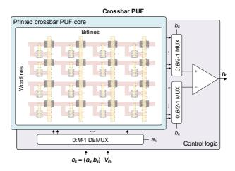
Figure 5.7: Printed crossbar PUF including addressing and readout schematic and PUF core. The diode-connected EGT crossbar builds the PUF core, whilst the external circuitry is the PUF control logic, which is required for CRP generation. Adapted from [219], © 2021 IEEE.
