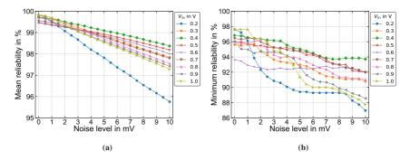
Figure 5.18: DiffC-PUF reliability over  $V_{in}$  and NL. (a) Mean reliability. (b) Minimum reliability. Adapted from [129],  $\bigcirc$  2019 IEEE.
