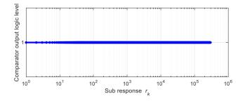
Figure 6.3: Comparator output, over the corresponding 298, 200 sub-responses  $r_k$ , during the prolonged continuous cycling test.
