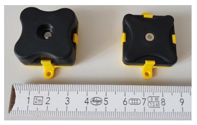
Figure 5. Teraranger Thermal 33 and 90.
