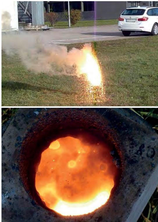
Fig. 2: Thermite reaction (left top) to 88 g of liquid iron (left bottom)
