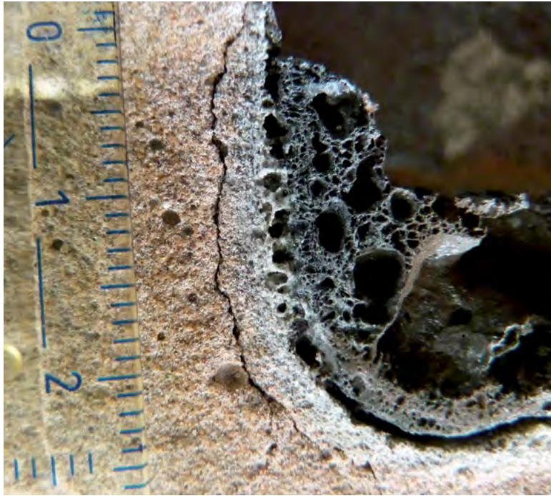
Fig. 4: Enlargement of the contact area between the mold and the molten iron
