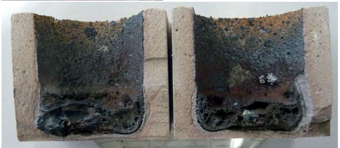
Fig. 3: Image of the mold cut open in the middle (external dimensions: 10 cm x 10 cm x 10 cm)
