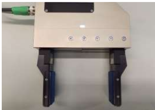
Fig. 1. Electrical Gripper from Weiss Robotics
