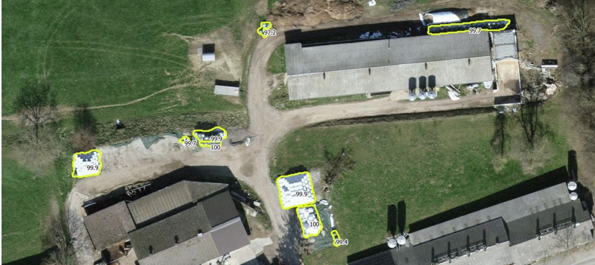
Fig. 5: Raw inference detections (yellow) of silage bale stacks displaying very high confidence scores outside of the TRN/VAL/TST subsets.
