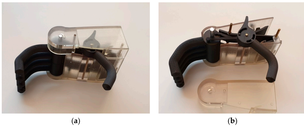
Figure 3. Second 3D-printed polymer replica of the first “Iron Hand” of Götz von Berlichingen with an improved thumb lever mechanism. (a) General view of the artificial prosthetic hand; (b) view after removal of the lateral chassis cover with insight into the new mechanics.
