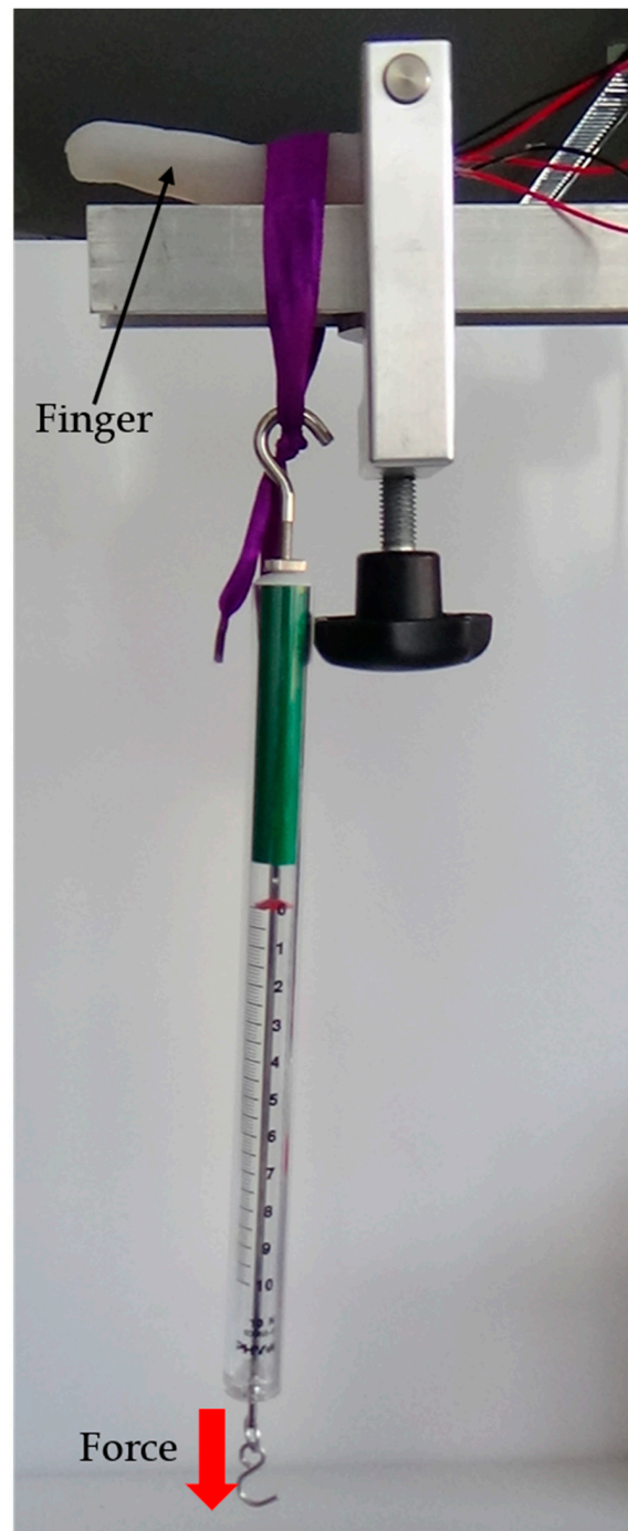
Figure 11. Measurement setup to analyze the force sensor. Force is applied to the proximal sensor using a flexible (purple) band.
