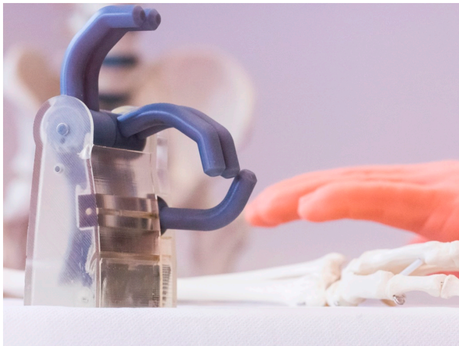
Figure 2. Initial 3D-printed polymer replica of the first “Iron Hand” of Götz von Berlichingen.
