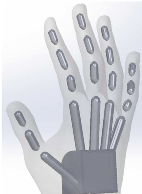
Figure 2. CAD model of the skeleton from simplified phalanges, which is placed inside the replacement hand.
