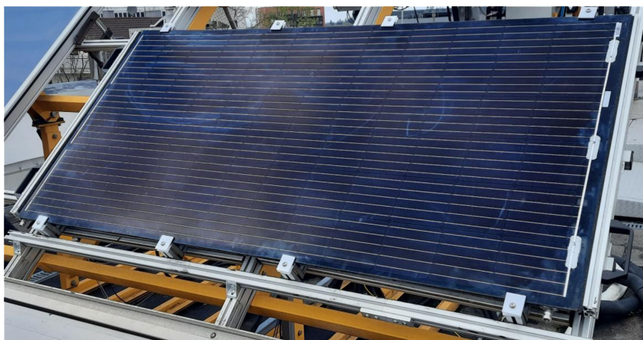
Figure 9. Finalized PVT collector prototype during characterization mounted on a solar test facility at the TestLab Solar Thermal Systems. Reproduced with permission. [31] Copyright 2022, Fraunhofer ISE.
