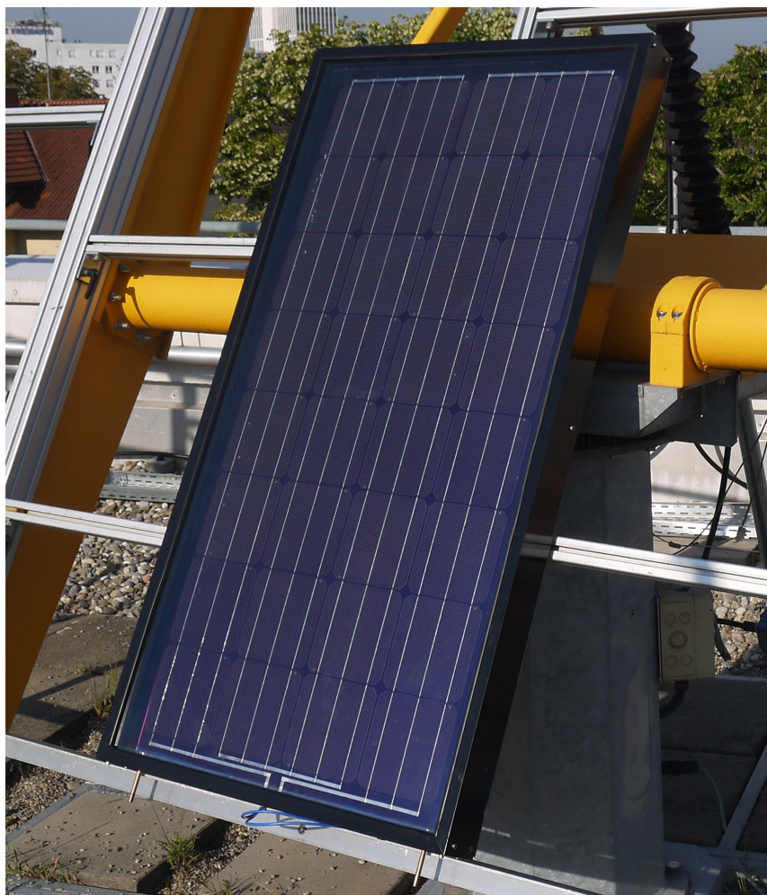
Figure 11. Covered PVT collector with low-e glazing during performance test on the outdoor test rig of TestLab Solar Thermal Systems at Fraunhofer ISE. Reproduced with permission. [31] Copyright 2022, Fraunhofer ISE.
