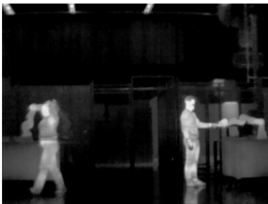
Figure 2. Infrared image in industrial settings with two cobots, a walking human on the left and a human interacting by hand guiding the cobot (R2) on the right (adapted from Süme et al., 2024a).
