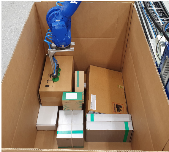
Fig. 2: Experimental setup of the robot performing a grasp in a bin with multiple objects with uneven center-of-mass
