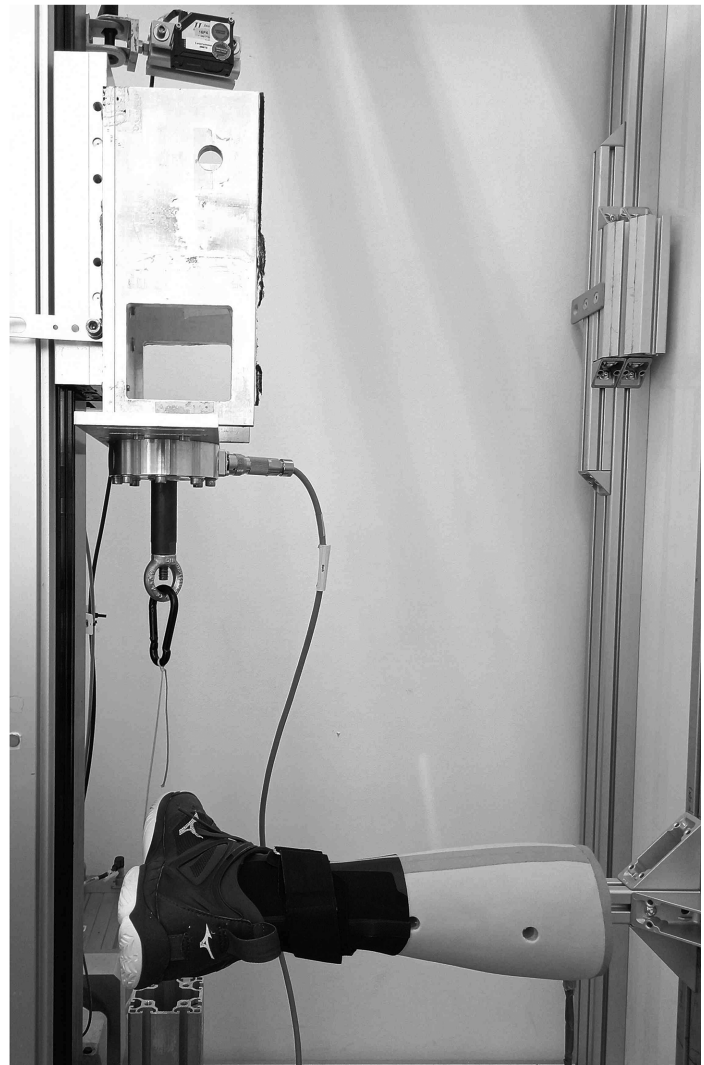
Figure 1. Mechanical tests performed with the artificial ankle (representing the right lower leg and foot) on the different brace conditions. Inversion is induced by pulling the rope connected to the lateral aspect of the foot upward. All braces were tested with the same shoe as during the biomechanical testing. Results represent the mean of 3 trials per condition.
