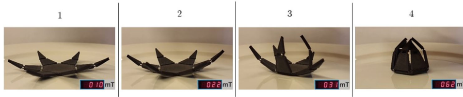
Fig. 9 Without an external magnetic field H , the star gripper remains at rest. With the appearance of the external magnetic field H , the star gripper bends to actuation structure. Especially, picture 3 shows the
